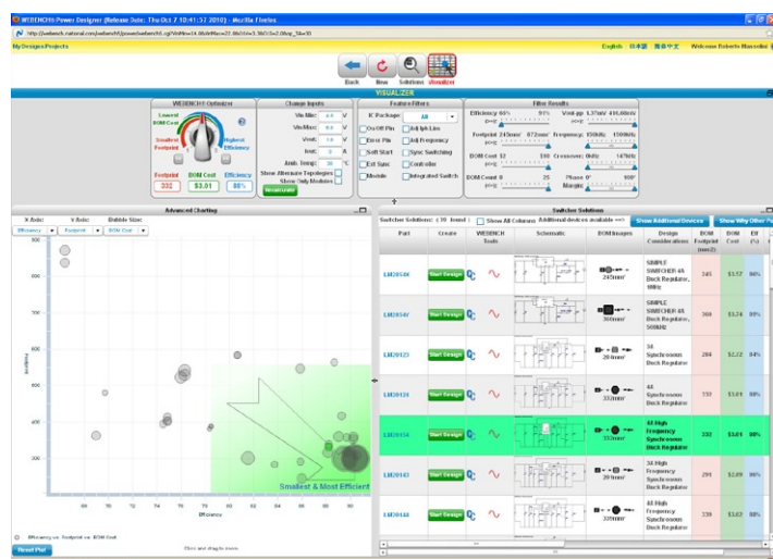
Fig. 3. WEBENCH allows the initial selection of the power converter, showing at glance the trade-off between cost, size and efficiency.
