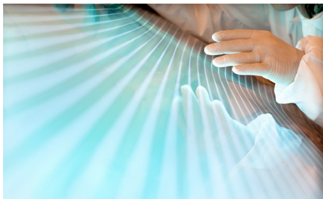
Konarka's Power Plastic® semi-transparent photovoltaic sheets can be used to laminate glass walls. Credit George Disario.
