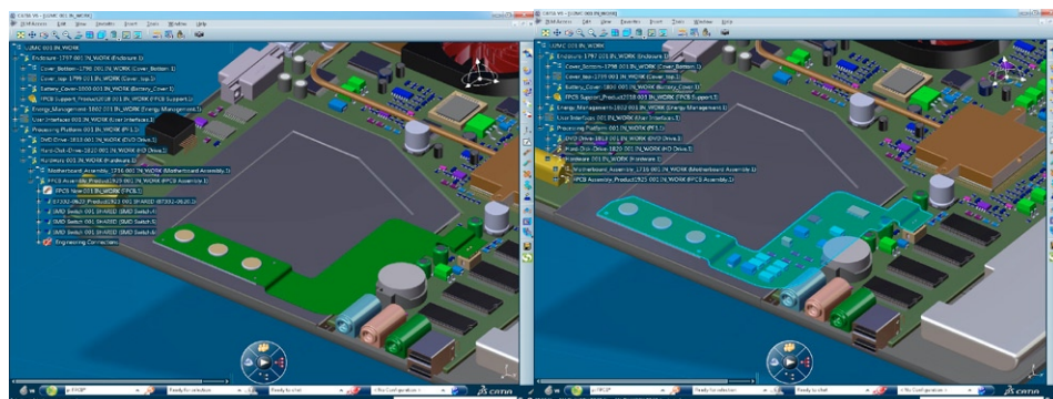
Fig. 2: Critical components are placed in 3D to ensure they respect the mechanical design constraints.
