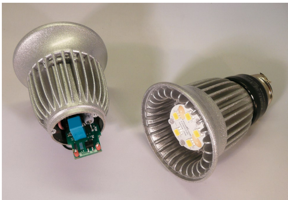
Fig. 1: A light bulb replacement has little room for a power supply.
